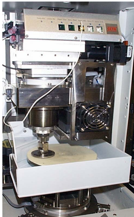
Fig.2: CMP Tester model PMT from Center for Tribology Inc.
