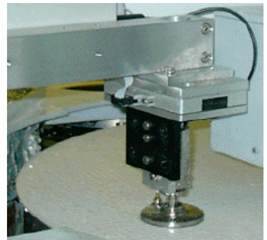
Fig. 14: PadProbe™ instrument for in-situ COF measurements
