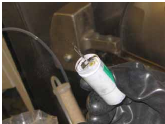
Cathode side of the jelly roll
